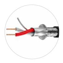
Data cable for transmission of DMX signals or for transmission of digital audio signals in AES/EBU format. Double shielding with spiral copper strands and an additional conductive foil shield for optimum resistance to interference, yet the cable remains highly flexible and rugged. Equipped with 3-pin XLR connectors by REAN ©.
