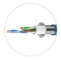
This EtherSound compatible CAT5e cable uses a highly flexible low smoke zero halogen jacket and braid shield of 128 tinned copper strands with four twisted pairs of conductors. It is terminated with rugged industrial grade RJ 45 connectors.
