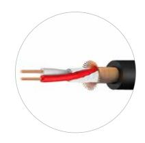
Balanced microphone or signal cable, equipped, like all cables in the K4MFP series, with female XLR plugs and 6.3 mm TRS stereo plugs by REAN © - making it the ideal choice for transmitting microphone signals to the board. The highly flexible cable has a braided shield and thus guarantees interference-free signal transmission.
